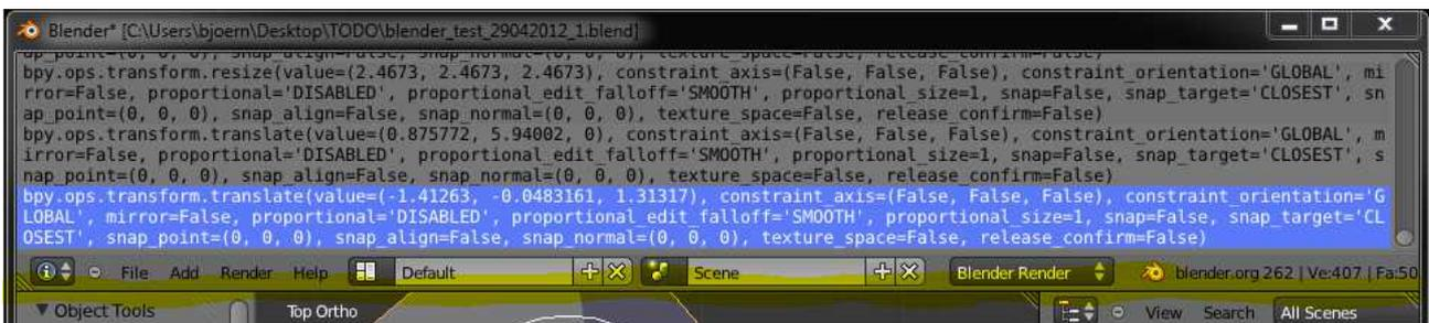
The Python-Scripts executed by Blender are always shown in the top section which is normally hidden. To open this section, the yellow marked line (see screen shot) has to be dragged down with the Mouse+LeftPress.
